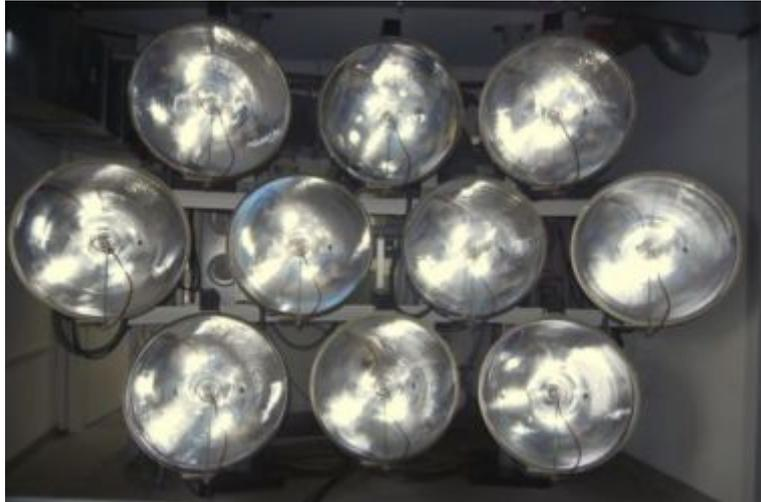
**Figure 4:** DLR High Flux Solar Simulator
