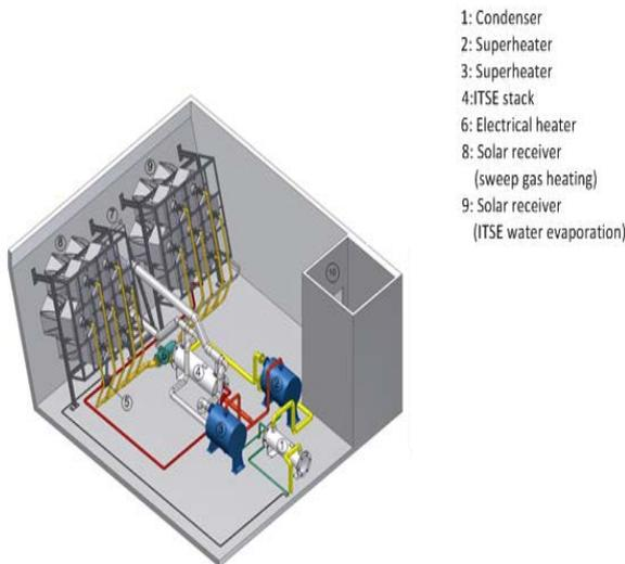
Figure 10a: design of the demonstration plant
