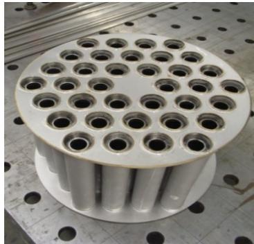
**Figure 11:** Steam generator (HyGear)
