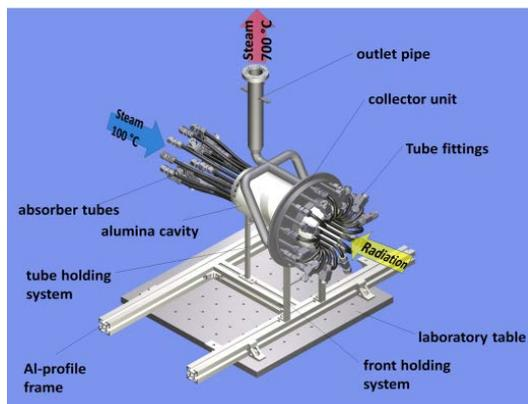
**Figure 6:** CAD design of the SoHTEK receiver
