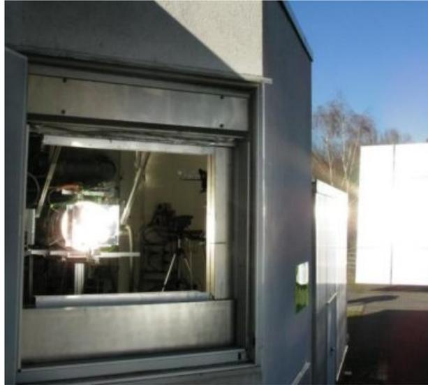
**Figure 3:** Shutter of the solar furnace
