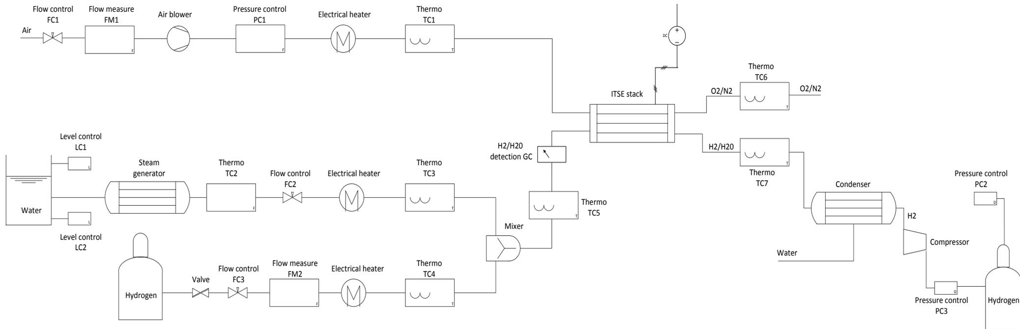
**Figure 8:** Flow sheet of the demonstrator in the laboratory
